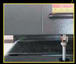
The self-centering and selftensioning conveyor belt will adjust to keep output media neatly stacked.
